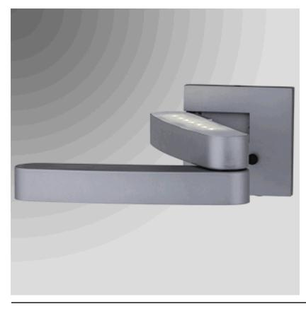
4.93"H Silver Alumnium Integrated LED Right Side Hinged Wall Lamp, seven 1.2 watt uplight with 120° beam, one 3 watt downlight with 15° beam, 402 total lumens, 4100K, direct wired, 4-way switch, with diffused lens cover
